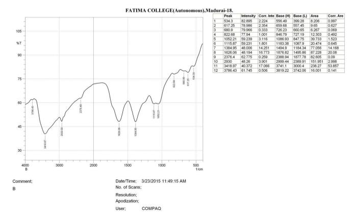
**Figure 6.** FTIR spectra of *Ipomoea pes-tigridis* synthesized silver nanoparticles.
