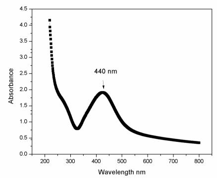
**Figure 2.** UV-vis spectra of *Ipomoea pes-tigridis* synthesized silver nanoparticles.
