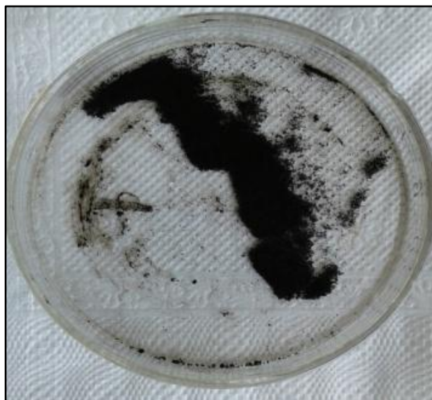
Figure 2. Gram-scale well-soluble hydrophilic \text{Fe}_3\text{O}_4 NPs were prepared by chemical coprecipitation method. (a) Samples of solid state hydrophilic magnetic nanoparticles powder on a Petri plate. (b) Dispersion in water, which can be moved by a magnet.
