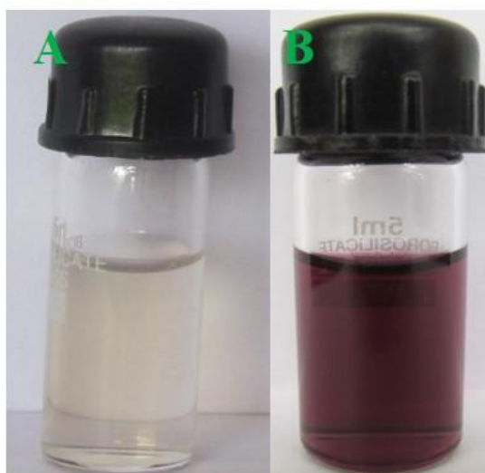
Figure 1. Color change profile of biosynthesized gold nanoparticles.
