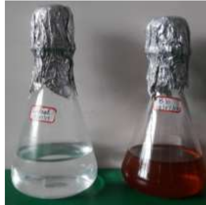
Brown Coloured Reaction Mixture of Beauveria bassiana obtained During Biosynthesis of Silver Nanoparticles.
