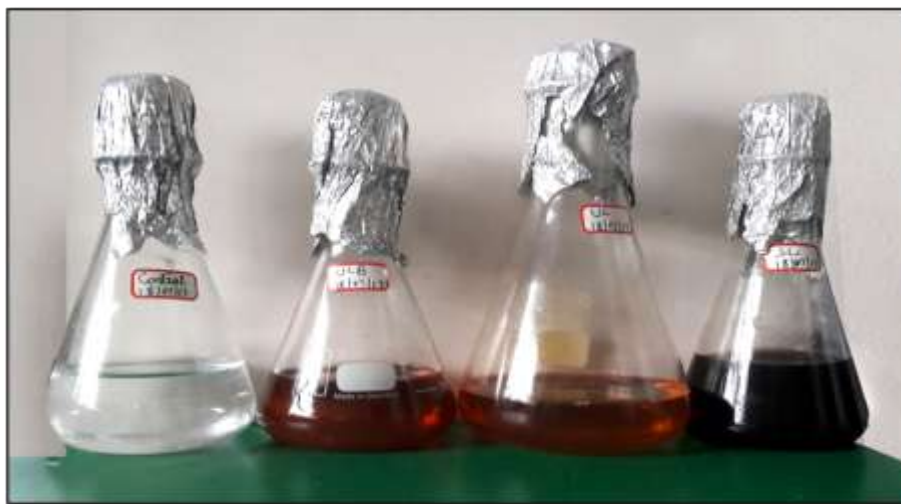
Figure 3. Brown Coloured Reaction Mixtures of 3 Endophytic Fungal Isolates obtained during screening for Biosynthesis of Silver Nanoparticles.
