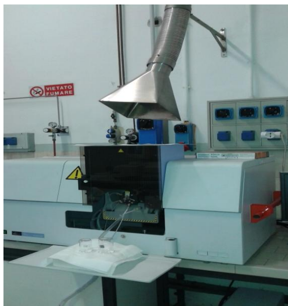
Figure 2. Perkins-Elmer Analyst 800 atomic absorption spectrometer used for mineral analysis.
