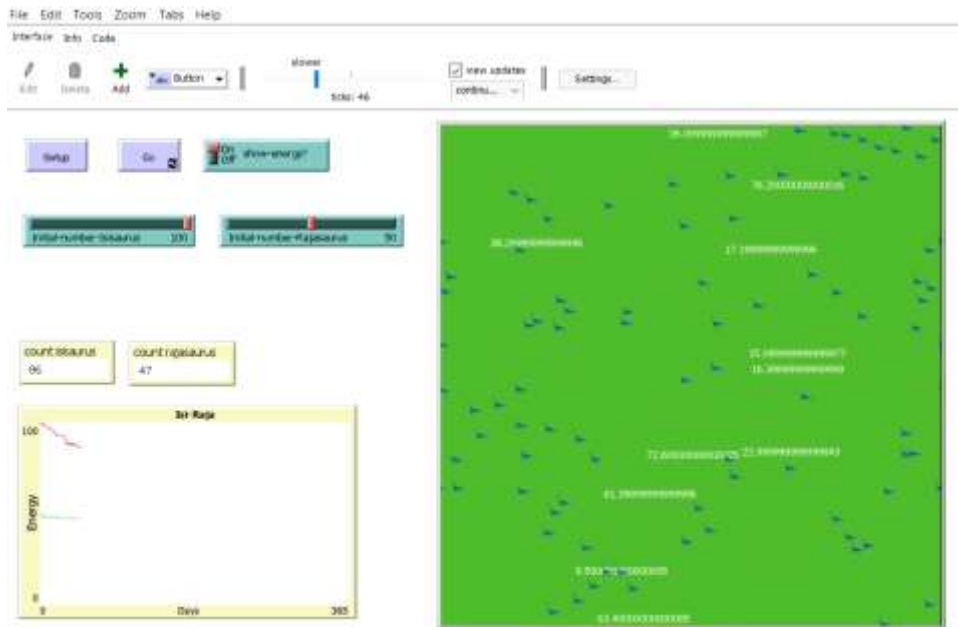
Figure 1. Interface of Netlogo program displaying the simulation space with programmed agents and parameter controls.
