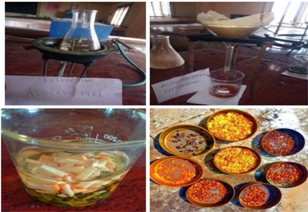
Figure 1. Processing of Raw materials (a) Extraction (b) Filtration (c) Washing (d)Drying.
