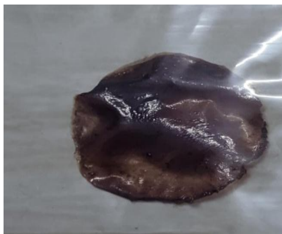
Figure 2. The highest conducting \text{NaClO}_4 -doped Areca catechu polysaccharide (SBE) film.
